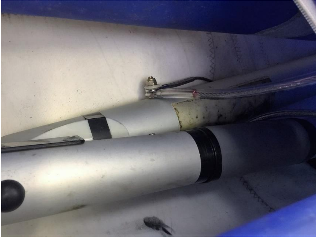
Cross-tube end of the side wires.
